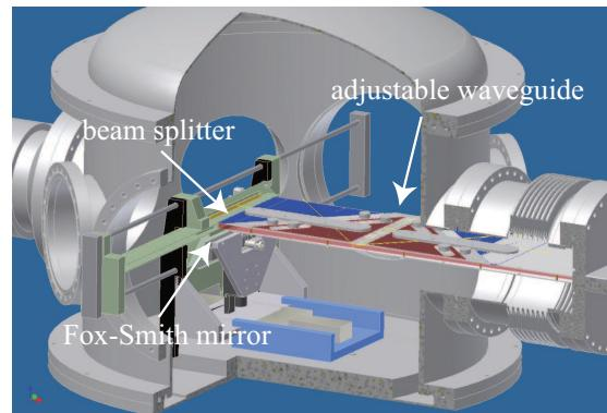
Figure 3: Design of the upstream mirror system, visible through a cut through the vacuum chamber. Left the Fox-Smith interferometer system with removable beam splitter. Right (in blue and red) the adjustable part of the waveguide required to allow cavity detuning over a 2-3 cm range.
