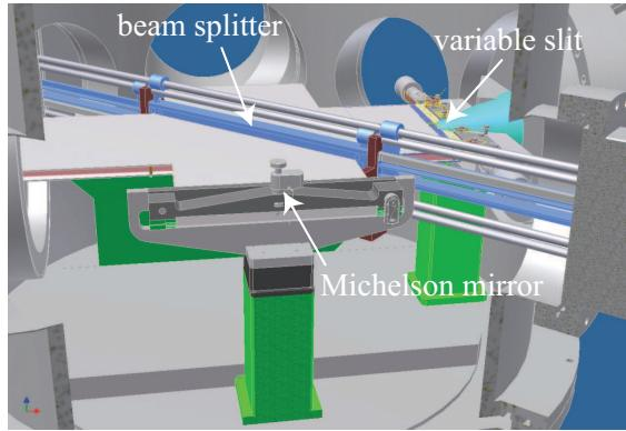
Figure 4: Design of the downstream mirror system. Right: adjustable vertical slit output coupler. Front: Mirror of the optional Michelson interferometer output coupler. The prominent mechanism is for the removable beam splitter of the optional Michelson interferometer.
