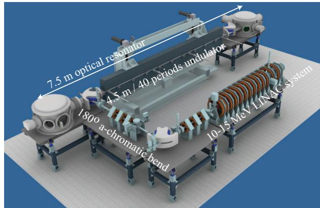
Figure 1: 3D design of the Nijmegen THz-FEL, showing LINAC, electron beam transport system, and optical cavity including 4.5 m long undulator.
