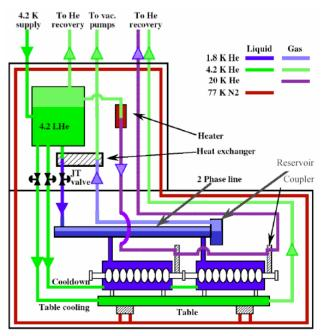
Figure 3: HOBICAT cryogenics.
