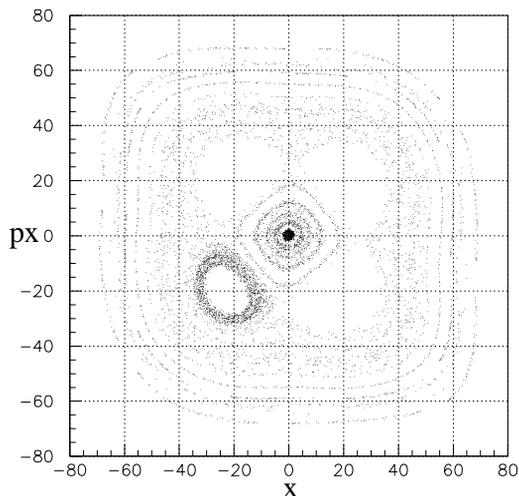
Figure 4: A horizontal phase space plot of 20 test particles for 400 turns when the intensity was  $8 \times 10^{11}$  ppb and the horizontal tune was 7.05.
