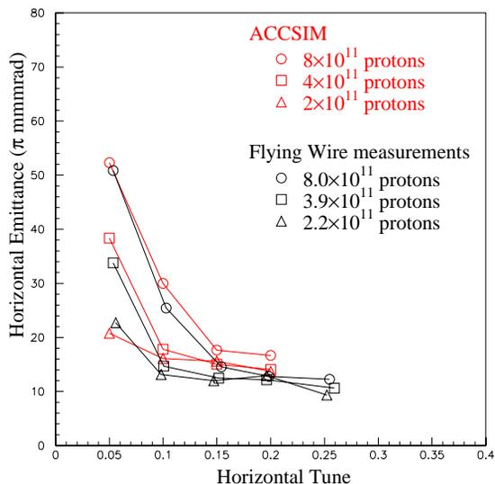
Figure 5: Horizontal 87 % emittance as a function of the horizontal tune when the intensity was 2, 4 and  $8 \times 10^{11}$  ppb. Flying wire measurements are shown in black symbols and results from the ACCSIM simulation are in red symbols.
