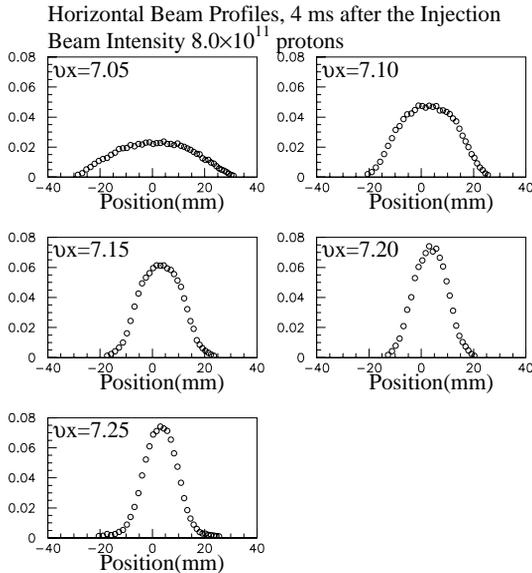
Figure 3: The horizontal beam profile 4 ms after the injection when the intensity was  $8 \times 10^{11}$  ppb and the horizontal tune was 7.05 ~ 7.25.
