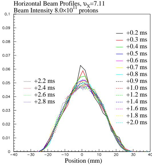
Figure 2: The horizontal beam profile 0.2 ~ 2.8 ms after the injection when the intensity was  $8 \times 10^{11}$  ppb and the horizontal tune was 7.11.
