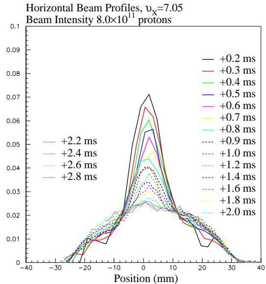
Figure 1: The horizontal beam profile 0.2 ~ 2.8 ms after the injection when the intensity was  $8 \times 10^{11}$  ppb and the horizontal tune was 7.05.
