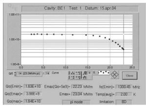
Figure 8: Test result of second prepared TESLA cavity BE2. No field emission was observed. The Q drop at highest fields is without indication of x-rays. The cavity was limited at 23 MV/m by a quench.
