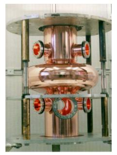
Figure 1: Single cell 400 MHz LHC cavity before sputtering with niobium.
