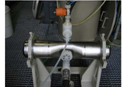
Figure 9: First HWR 176 MHz cavity during chemical treatment at ACCEL.
