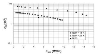
Figure 2: Typical result of a 400 MHz Nb/Cu plated cavity for LHC produced and prepared at ACCEL. The RF test was performed at CERN.
