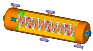
Figure 10: Cut view of the 352 MHz superconducting CH mode cavity.
