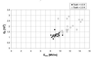
Figure 3: Highest gradients E<sub>acc</sub> and quality factors Q<sub>0</sub> at the highest gradients achieved at bath temperatures of 4.5 K and 2.5 K in the 21 LHC 400 MHz single cell cavities. The tests were carried out at CERN.
