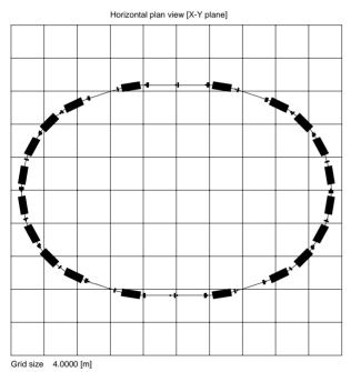
Figure 1. Footprint of the CLS Booster lattice.
