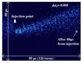
Figure 6: Double-sweep streak camera image with improper  $\alpha_2$ . The vertical axis is the rf phase of the ring and the horizontal axis is the revolution.
