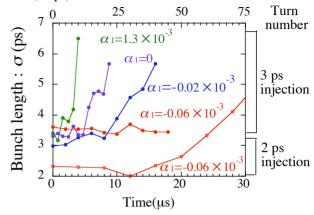
Figure 3: The elongation of the bunch length after injection for different values of  $\alpha_1$ . The initial length was not the shortest, because the buncher phase of the linac was not optimized at that time.
