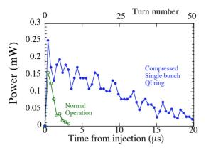
Figure 5: The turn-by-turn CSR power after injection. The line with open circles shows the power obtained with the parameters of normal operation, where there were three bunches in a pulse. The line with filled circles shows the power obtained from one compressed bunch in a QI ring. The bunch charge was about 20 pC/bunch in both cases.
