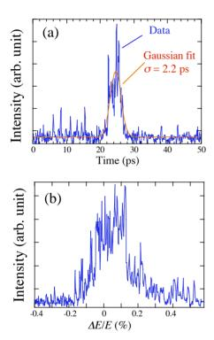
Figure 2: Time profile (a) and energy distribution (b) of the compressed linac bunch measured at BL6.
