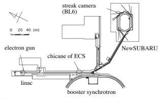
Figure 1: Layout of the SPring-8 linear accelerator, the energy compression system (ECS), the booster synchrotron, and the NewSUBARU storage ring. The streak camera is placed in beamline 6 (BL6) of NewSUBARU.
