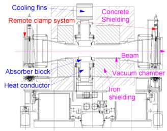
Figure 1. Schematic of J-PARC RCS collimator
