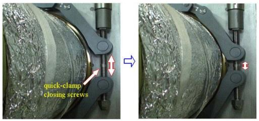
Figure 7. Close the quick-coupling clamp
