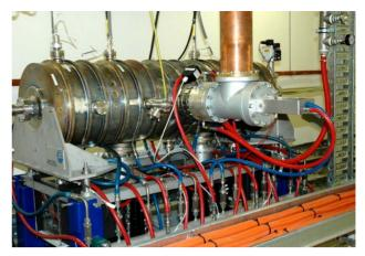
Figure 3: ASP Booster Cavity after installation.
