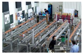
Figure 1: Linac functional units. In the front: accelerating structures during tuning, in the back left: MEBT; in the back right : bunching section during assembly.
