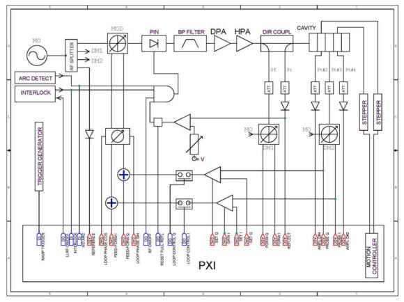
Figure 4: ASP booster LLRF diagram.
