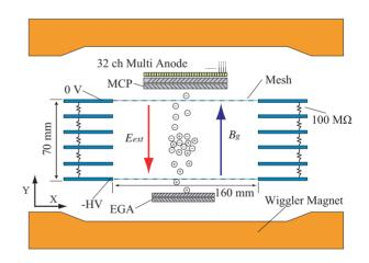
Figure 1: Cross section view of the prototype.
