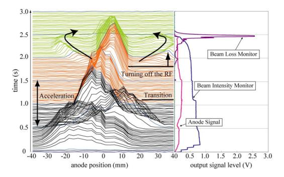
Figure 2: Mountain view of the obtained profiles for the ion collection mode (left). Raw signals from the MCP central anode (-1.25 mm from the center), a beam intensity monitor, and a beam loss monitor are also shown (right).
