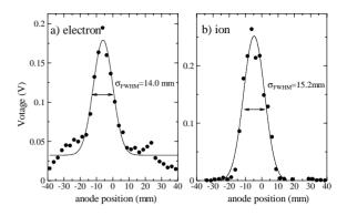
Figure 3: Typical beam profiles obtained at just before the transition energy, 1 s after the injection, for electron collection mode a) and for ion collection mode b). The solid lines are the fitted results.
