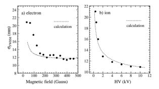
Figure 4: The dependences of measured beam sizes on the guiding field for the electron collection mode a) and on the applied HV for the ion collection mode b). The dashed lines are the calculated results.
