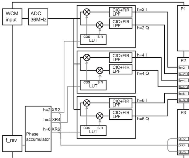
Figure 1: BCA (Beam Current Analysis) module, main part.
