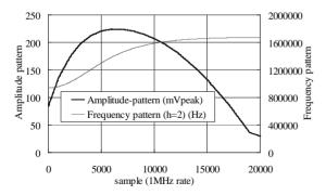
Figure 5: The 20 ms acceleration part of the RCS ramp.
