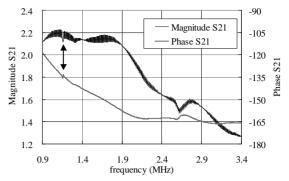
Figure 6: S21 transfer function of the RCS high power system measured between driver amplifier input and differential signal of both capacitive gap voltage dividers.
