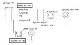
Figure. 3: DSP+DDS Combination for high power tests.
