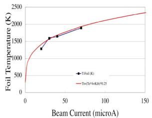
Figure 6: Foil temperatyre v. s, dc beam current
