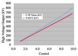
Figure3: The terminal voltage of ion source v. s. the nominal C-W output voltage.
