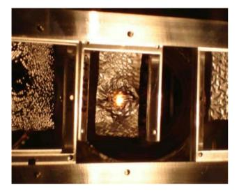
Figyre 5: An example of beam spot on the carbon foil.
