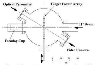
Figure 4::Layout of the target chamber with multiple target folders.
