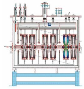
Figure 4: Prototype superconducting module containing six superconducting half wave resonators ( $\beta$ =0.09) and three superconducting solenoids.
