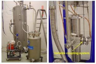
Figure 5: Vertical test facility at ACCEL. The cryostat (left) is filled with helium out of dewars and pre-cooled with  $LN_2$ . The superconducting half-wave resonator is equipped with a variable input coupler for the vertical test (bottom).
