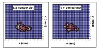
Figure 3: Beam emittance measurement ( $\varepsilon_{norm,rms,100\%} = 0.15 \pi$  mm mrad at 5 mA H+).
