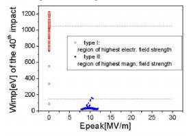
Figure 8: Calculated impact energy of the 40<sup>th</sup> electron for the two kind trajectories shown in figure 7.
