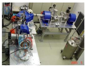
Figure 1: ECR Ion Source with LEBT in the ACCEL test facility.
