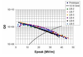
Figure 6: Test results of the half wave resonators produced for the SARAF linac.
