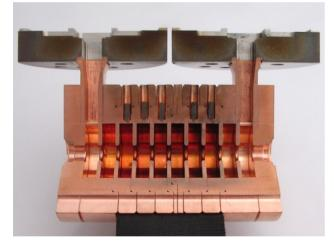
Figure 2: A cross-section of deflecting cavity prototype.
