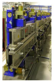
Figure 2: Picture of the SPARC undulator chain during installation.
