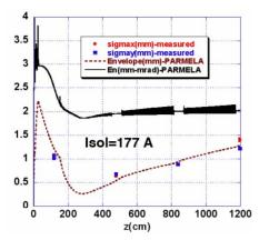
Figure 4: PARMELA simulation of the envelope and emittance corresponding to the best measurement shown in Fig. 3. The measured enevelopes (blue rectangle) are also shown.
