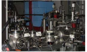
Figure 5: Harmonic generation chamber in the SPARC Hall.
