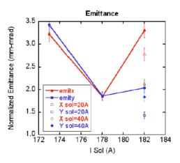
Figure 3: Emittance measurement for different configuration of the gun solenoid and the coils around the accelerating structures.
