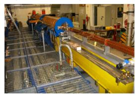
Figure 1: Picture of the SPARC photoinjector showing t3 accelerating structures with 2 long solenoids.
