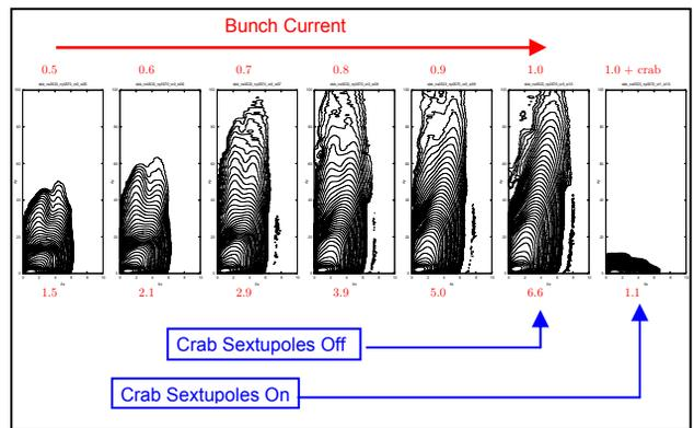
Figure 6: Beam tails and vertical blowup (numbers at the bottom) vs. bunch current and Crab Waist.
