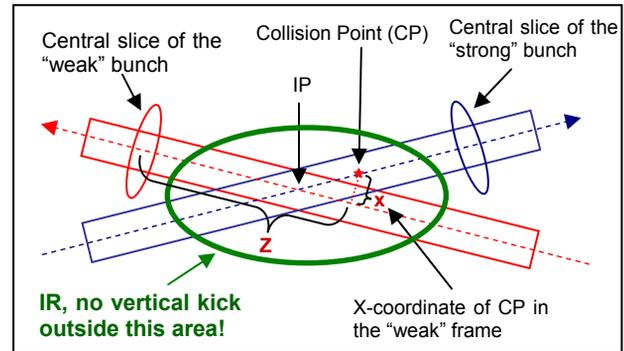
Figure 3: Collision with large Piwinski angle.
