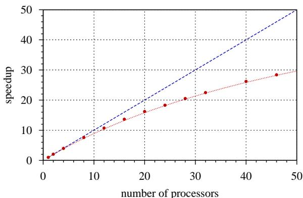
Figure 3: Speedup achieved by running Astra on multiple processors. The dashed line indicates the ideal case of full scalability, the dotted line corresponds to Amdahl’s law with a sequential code fraction of  $\alpha = 1.4\%$ .
