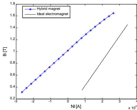
Figure 6: Characteristics for an optimized hybrid magnet and an ideal electromagnet.
