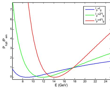
Figure 1: The ratio of the power of a conventional electromagnet and a hybrid magnet with the same geometry as function of beam energy. The hybrid magnet is favoured for ratios lower than 1.
