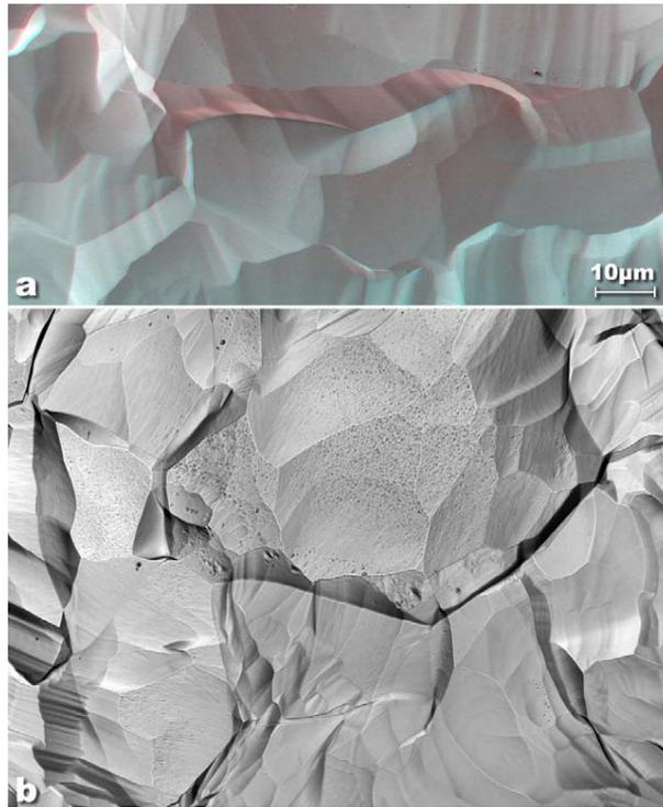
Figure 3: a) 3D red-blue anaglyph FESEM image and b) Laser Confocal Microscope (Olympus LEXT) courtesy Erich Zeiss of Leeds Precision Instruments). Images at similar magnification of BCP etched surface representative of the FNAL cavities.
