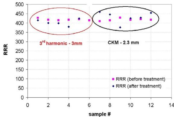
Figure 4: RRR for material used in the fabrication of prototype 3<sup>rd</sup> harmonic and transverse deflecting cavities.
