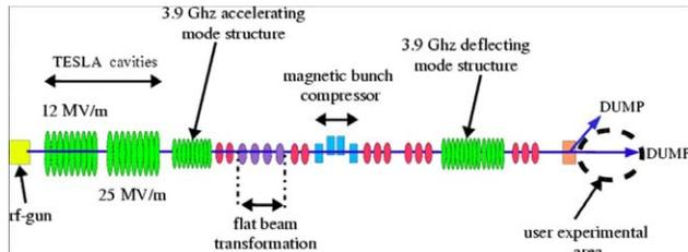
Figure 1: Upgraded A0 facility beam line layout.
