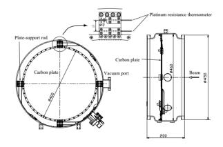
Figure 1: Shematic drawing of the BIHM.
