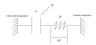
Figure 2: Equivalent circuit of the BIHM.
