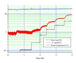
Figure 3: Responce of the sum of the four  $\Delta T$  signals to the heat loads and room temperature.
