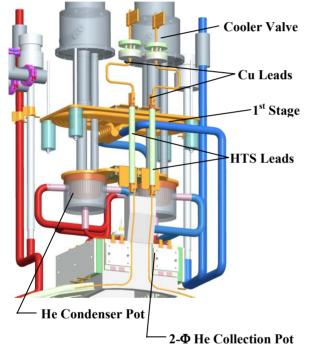
Figure 4. Coupling Magnet Neck Assembly
