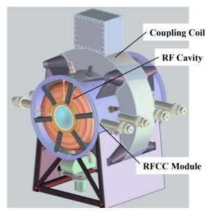
Figure 1. The RFCC Module and Coupling Magnet
