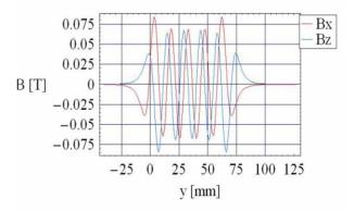
Figure 4: Simulation of the magnetic field in undulator.
