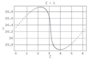
Figure 5: Genesis simulation of the energy-phase modulation after 30 cm drift.
