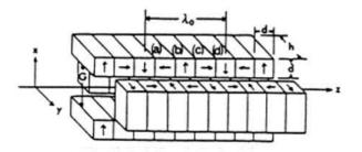
Figure 3: Undulator schematics. Arrows indicate the direction of magnetic field.
