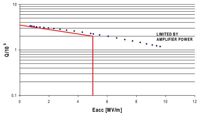
Figure 1: Typical cavity performance and acceptance curve
