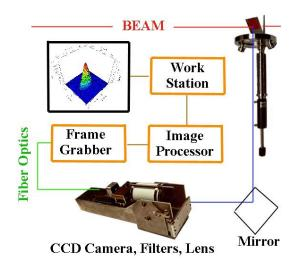
Figure 1: Beam Profile Monitor System
