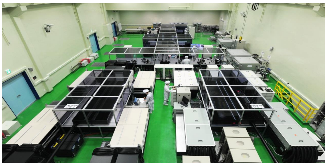
- 30-fs, 1-PW and 1.5-PW Ti:sapphire Laser operating at CoReLS -
