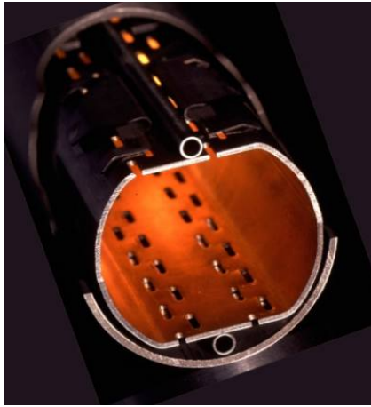
Figure 5.2: A sliced beam pipe from the LHC, with a rectellipse-like beam screen . Along the straight parts on top and bottom there are cooling pipes with liquid helium too ensure that the magnets nearby are not heated with the energy absorbed by the pipe. [8]
