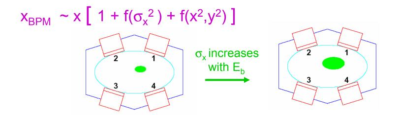
Biases change with energy and from BPM to BPM! Solution: take care to steer beam close to centre of BPMs and keep in same place for reference and high energy measurement
