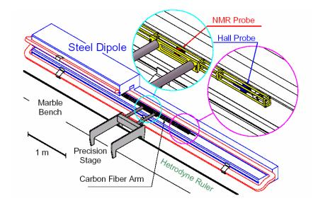
Measurements made by moving arm carrying NMR probe for core field, Hall probe for end fields
