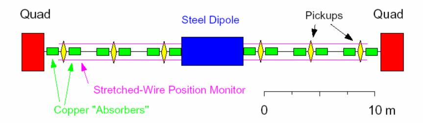
Required precision on position measurements ~ 1 micron; on  $\int B.dl ~ 10^{-5}$ . Recall these accuracies must be attained on measurements of *changes* between reference & high energy
