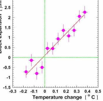
Residual expansions (5.5 microns / ° C) and movements followed by stretched wire sensors
