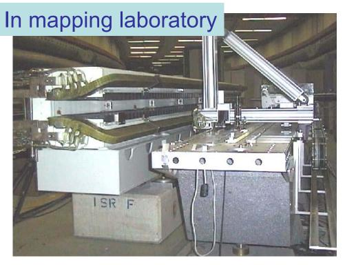
Local field measurements come from 4 NMR probes positioned on precision mounts
