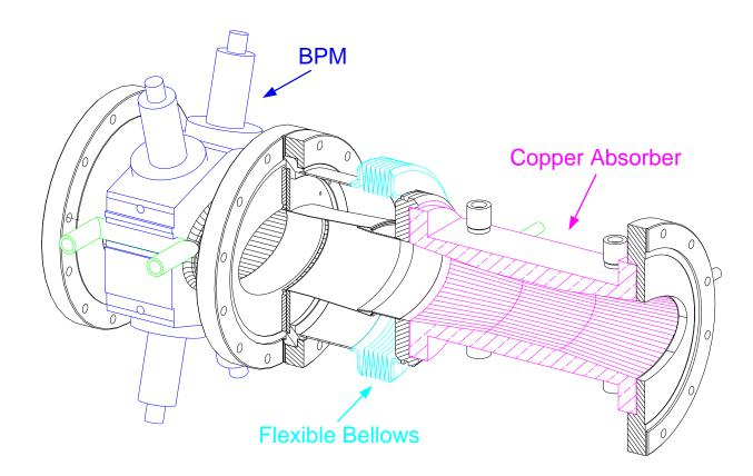
BPMs stable to  $<0.2^{\circ}C \rightarrow$  block expansion  $<1.5 \mu m$
