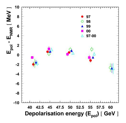
It works & is stable! However, how does above 'banana' evolve to 100 GeV, & is sampling representative of total  $\oint B \cdot dl$  ?
