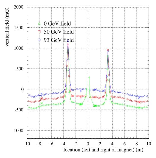
(Spikes come from permanent magnets in vacuum pumps. Energy variation from currents in magnet cables.)
