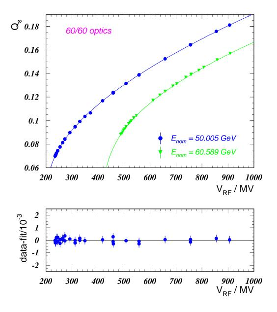
$\rightarrow E_b$  at 80 GeV with an error of  $< 2 \times 10^{-4}$ :
