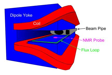
NMRs used in defining energy model, & flux loop to set error
