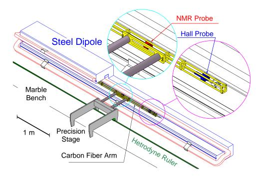
Model developed to relate  $\oint B \cdot dl$  to values of 4 reference NMRs in dipole as function of coil temperature etc
