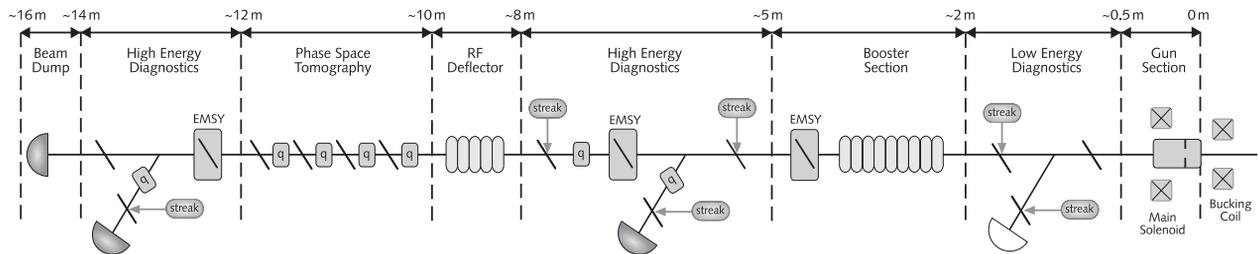
Figure 5: Preliminary layout scheme of the PITZ2 setup.
