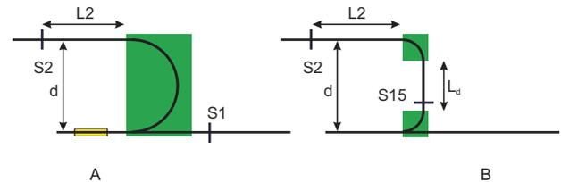
Figure 6: Two spectrometer setups under discussion. (A) A 180° dipole magnet followed by a drift space  $L_2$ . (B) Two 90° dipole magnets separated by a drift space  $L_d$  and followed by a drift space  $L_2$ .
