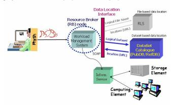
Fig. 1. Description of the analysis job submission in Grid. The user on the UI provides dataset and private code. The Workload Management System discovers the data location, via the Data Location interface to several catalogues, and submits the jobs on resources hosting the data.
