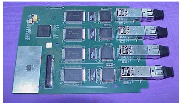
Figure 8 The 4TX board for sending simulated event data to the ROD. There is one 512KB SRAM per link for holding events. The control FPGA is on the left.
