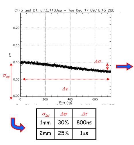
• Simulation with LSP show an electron focusing 4 times slower than the theoretical model.
