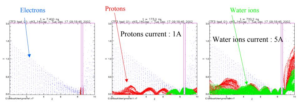
Based on the experimental observations done in the US and in France, two different kind of ions simulated : Protons 9%, OH<sup>+</sup> 91%
