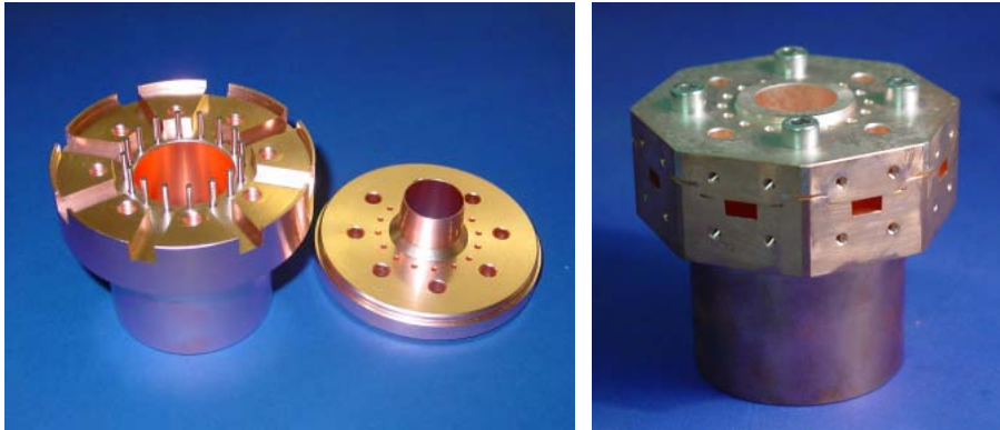
CLIC PETS Power extractor test set-up
