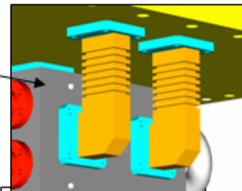
Waveguides in vacuum can with mitre bends
