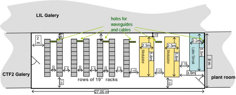
Enough space for all power supplies, vacuum, controls and beam diagnostics racks needed for CLEX beamlines
