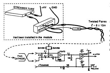
Fig. 4: Electronics for the read-out of one tube
