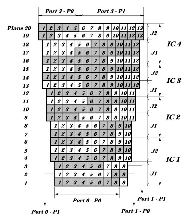
Figure 2.4: One module information read-out scheme
