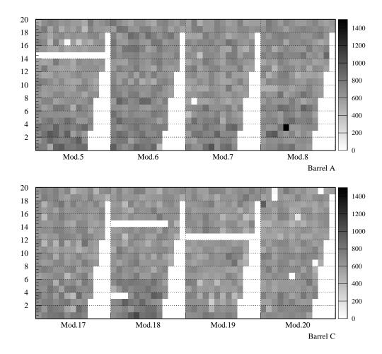
Figure 2.5: Tubes occupation chart. For each module, integrated number of hits in every tube is shown.
