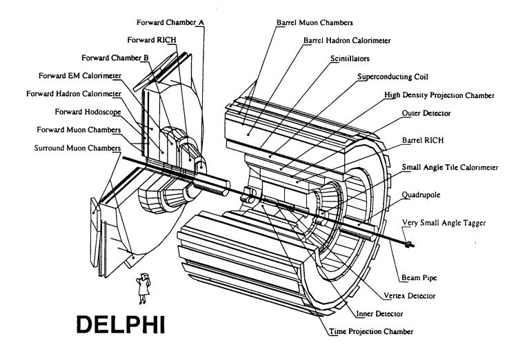
Fig. 1: The DELPHI detector
