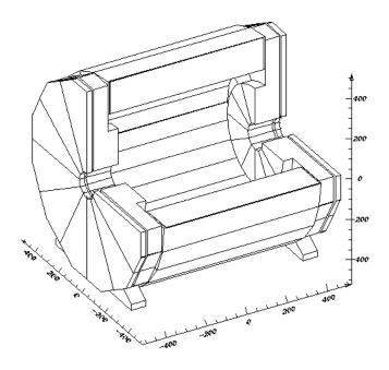
Figure 2.1: DELPHI Hadron Calorimeter
