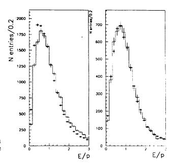
Fig 4: E/P ratio charged tracks with P<6 GeV (a) and P> 6 GeV (b) in Z decays. Here E is the full energy deposited and P the momentum of charged track. Data are shown by the points and simulation by the histogram
