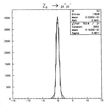
Fig. 8: Resolution of cathode read-out in φ direction
