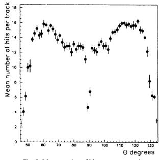
Fig. 8: Mean number of hits per muon track
