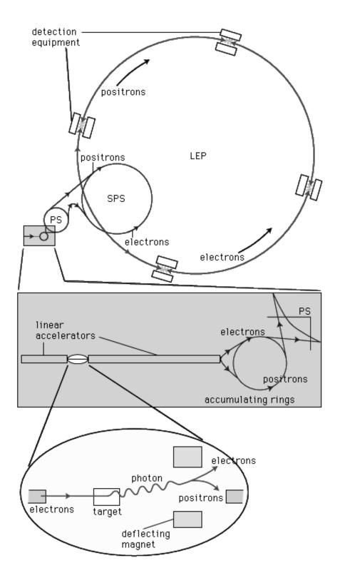
Figure 1.1: Scheme of the CERN accelerator complex
