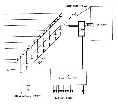
Fig. 14: Schematics of anode read-out
