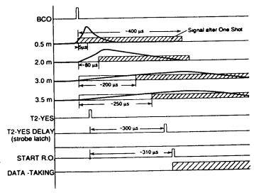
Fig. 3: Timing structure of HAC cathode signals
