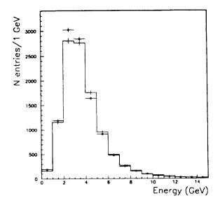
Fig. 2: Energy in HAC deposited by  $\mu$  identified in the  $\mu$  chambers (Fig. 1). Data (from the 1994 run) are shown by the points and simulation by the histogram
