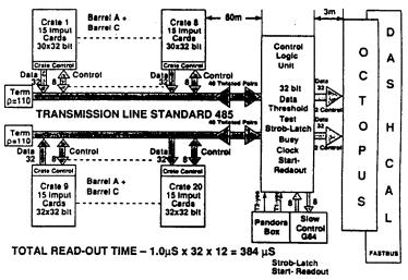
Fig. 5: Structure of the data transmission
