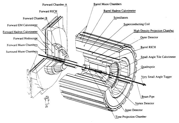
Fig. 1: The DELPHI detector
