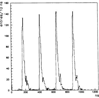
Fig. 15: Bunch structure in LEP seen by anode read-out
