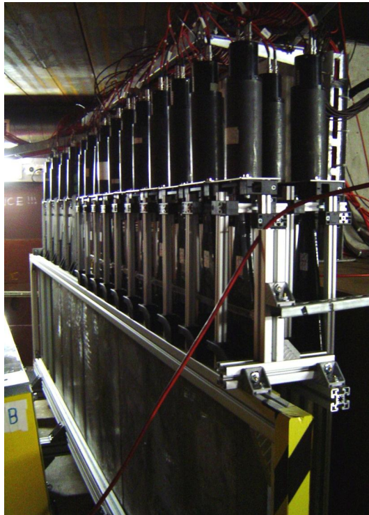
Figure 4. Preshower left arm in the DIRAC set-up
