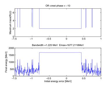
Figure 8: The maximum of Tr(R(z)) and the maximum achievable energy  $E_{max}$  along the length of the linac as a function of the arrival energy when the linac operates with -10 degree off-crest phase.
