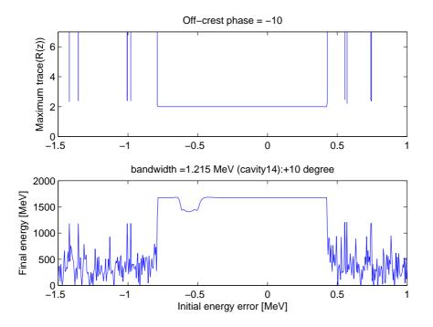
Figure 11: The transverse stability bandwidth of the linac operating at -10 degrees off-crest when cavity 14 is tuned to 0 degrees which means it operates oncrest. The stability bandwidth is determined from the Tr(R(z)) plot. Note that the maximum achievable energy in the lower graph has a pronounced dip at an energy offset of -0.5 MeV. This would cause part of the beam that has this offset to develop a tail with very low energy.
