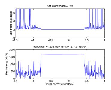
Figure 14: The energy bandwidth with a lattice where the focal length is chosen to be f = 15 m resulting in a weak transverse phase advance of 11.5 degree. Note that c, compared to Fig. 8 Tr(R) does not grow as quickly adjacent to the borders of stability at  $\pm 0.4$  MeV.
