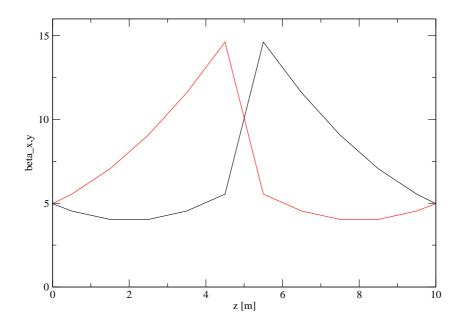
Figure 2: The horizontal and vertical beta functions between the cavities. The focal length of the thin lens quadrupoles is assumed to be f = 2 m giving a phase advance of 97.2 degree.
