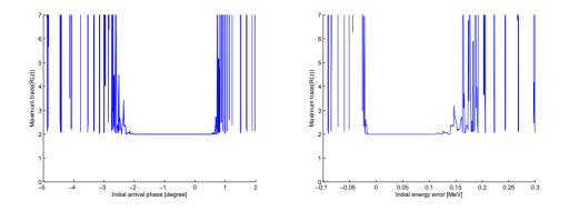
Figure 6: The maximum of Tr(R(z)) along the length of the linac as a function of the arrival phase (left) and the arrival energy (right).
