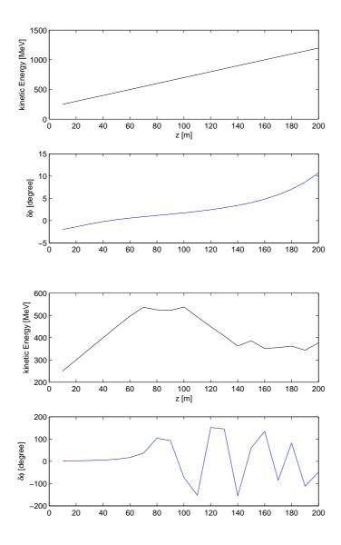
Figure 4: The energy profile along the length of the linac with an initial phase error of -2 degree (above) and +2 degree (below).
