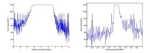
Figure 5: The energy at the end of the linac as a function of the initial phase offset (left) and offset in kinetic energy (right).
