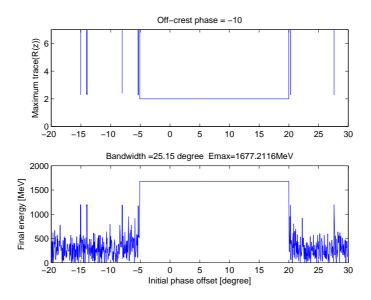
Figure 9: Max(Tr(R(z))) and  $E_{max}$  along the length of the linac as a function of the arrival phase when operating at  $\Delta \psi = -10$  degrees.
