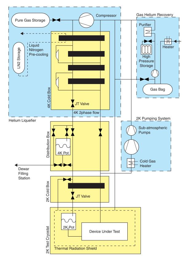
Figure 1: Layout of the helium cooling facility including a 2 K test cryostat.
