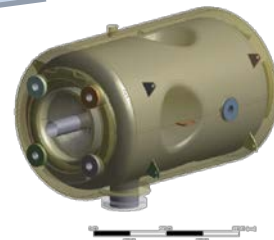
SRF Cavity (superconducting)
