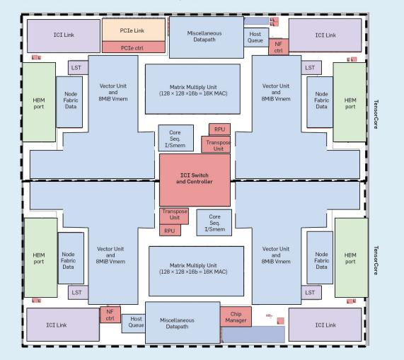
It has two TensorCores: Node fabric data and NF controller move on-chip data.
