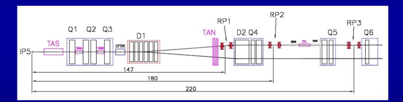
RPs at ~10 $\sigma$  imply : collimators must be set to 6/7 s. e<sup>\*</sup> ~ 1 mm, ~ 4 times smaller than nominal :
