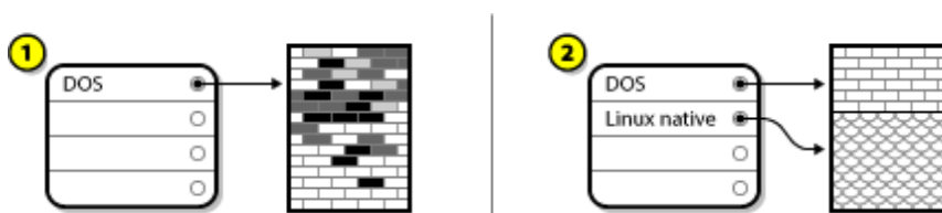
Figure A.10. Disk Drive Being Destructively Repartitioned
