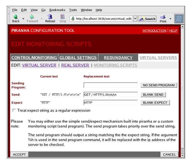
Figure 1.37. The EDIT MONITORING SCRIPTS Subsection
