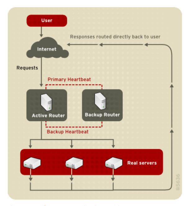
Figure 1.23. LVS Implemented with Direct Routing
