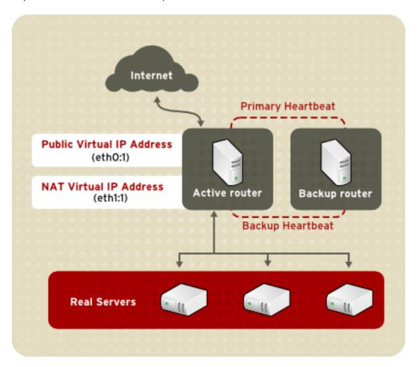
Figure 1.22. LVS Implemented with NAT Routing
