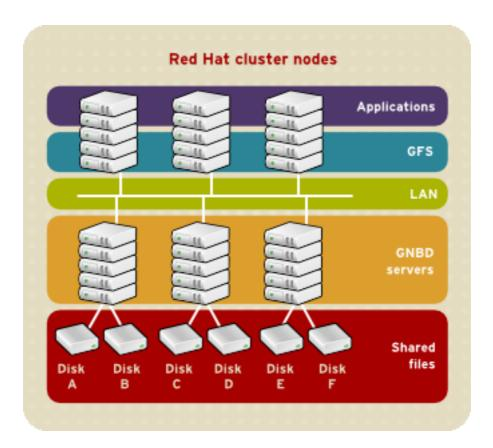
Figure 1.13. GFS and GNBD with Directly Connected Storage
