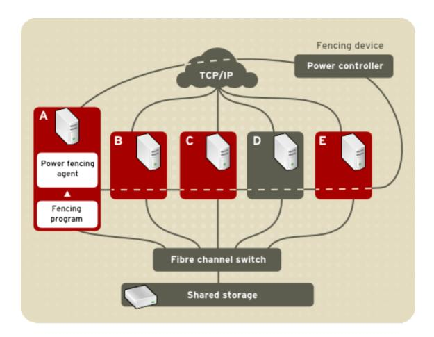
Figure 1.3. Power Fencing Example
