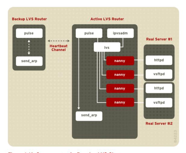
Figure 1.19. Components of a Running LVS Cluster
