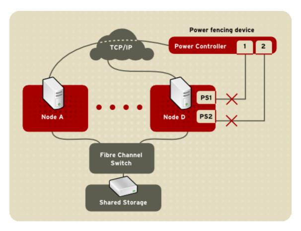
Figure 1.5. Fencing a Node with Dual Power Supplies
