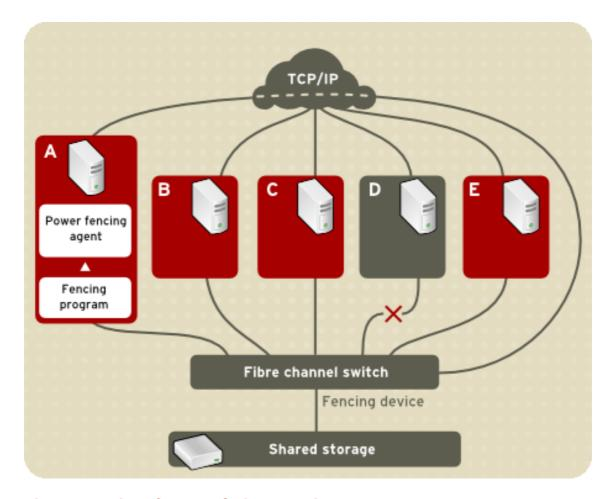
Figure 1.4. Fibre Channel Switch Fencing Example
