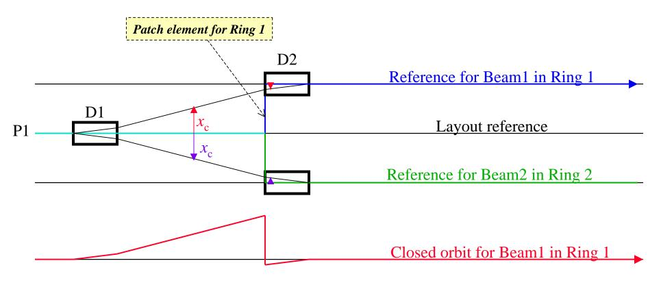
Both D1 and D2 have zero angle But K<sub>0</sub>= ±α/L to make closed orbit.
