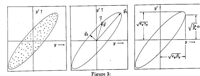
a) Particles occupying some area in phase space observed at some point in the lattice may be enclosed by an ellipse b) This ellipse is generated by two phase space vectors  $\vec{z}_1$  and  $\vec{z}_2$ . The motions of these generating vectors characterize the motion of all of these particles through the lattice. c) The resulting generating trajectories in turn can be expressed in terms of lattice functions which describe the shape of the phase ellipse everywhere in the
