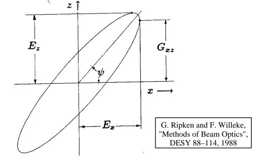
Figure 8: Projection of the four dimensional phase ellipsoid onto the x-z-plane
