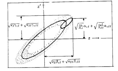
Figure 4: Two sets of lattice functions for each plane describe the projection of a four dimensional torus on the x - x' and y - y'-planes.
