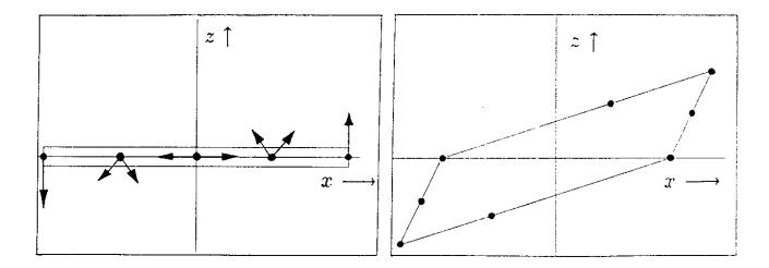
Figure 2: Effect of a skew quadrupole on a flat beam. The arrows indicate the slope of the particles behind the skew quadrupole (left). The beam is observed after some downstream drift behind the skew quadrupole. It is transformed into a parallelogram (right).
