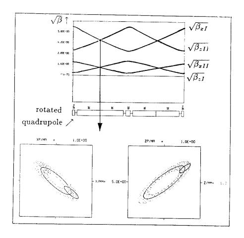
Figure 5: Coupled Lattice functions for a FODO-cell with a rotated quadrupole.
