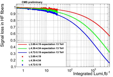
Expected loss of signal for up to 3000 fb<sup>-1</sup> In the highest  $\eta$  region, signal reduction by factor x3-x4 is expected and can be compensated by re-calibration. HF will survive 3000 fb<sup>-1</sup>, at least up to
