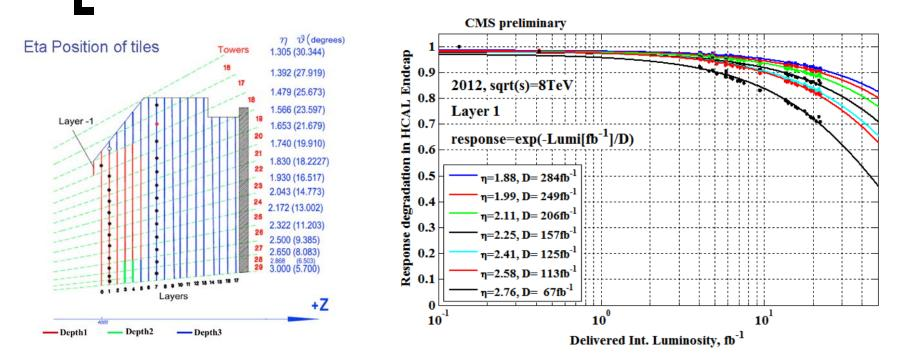
Degradation of signal (loss of scintillation and reduced transmission of light) in CMS HCAL Endcap in 2012 for the first sampling layer.
