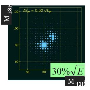
$\sigma_{Ejet}/E_{jet} \sim 3\%-4\% @ \sim 50 \text{ GeV} \rightarrow \sigma_{Ejet}/E_{jet} \sim 25-30\%/\sqrt{E}$
