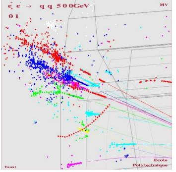
Emphasys on tracking capabilities of calorimeters Use granularity to correctly assign hits to showers 60% of jet energy measured with tracker 30% of jet energy measured in ECAL 10% of jet energy measured in HCAL
