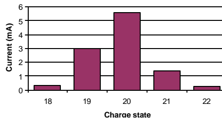
Figure 14. Current traversing the second slit as a function of charge-state.
