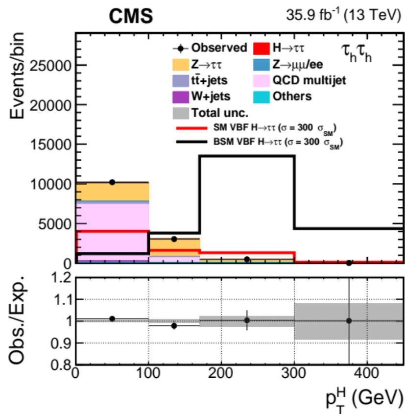
The distributions of transverse momentum of the H boson in the boosted category of the  $e\tau_h + \mu\tau_h + e\mu$  (left) and  $\tau_h \tau_h$  (right) decay channels. The BSM hypothesis corresponds to  $f_{a3} = 1$ .
